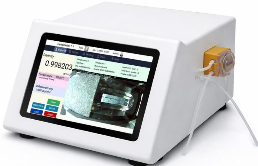
Automatic Density Meter is a high-precision analytical instrument engineered for fast, accurate, and repeatable measurement of liquid density.
